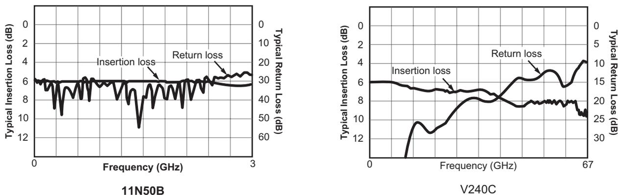
**Figure 3.** Return Loss and Insertion Loss (Typical)
