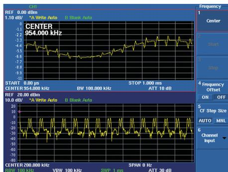
Inverter noise superimposed on broadcast waves
