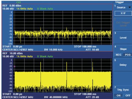
Local signal inside the mobile phone superimposed on broadcast waves
