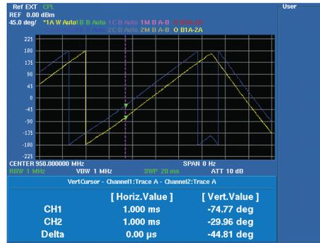
Measurement of phase difference (time difference) of 1/2 path
