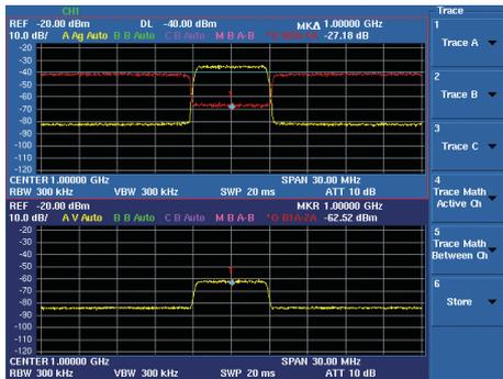
Horizontal polarized wave signal and XPD (difference between the vertical and horizontal polarized waves)
