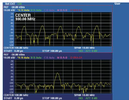
Magnetic field radiation from the electronic component surface
