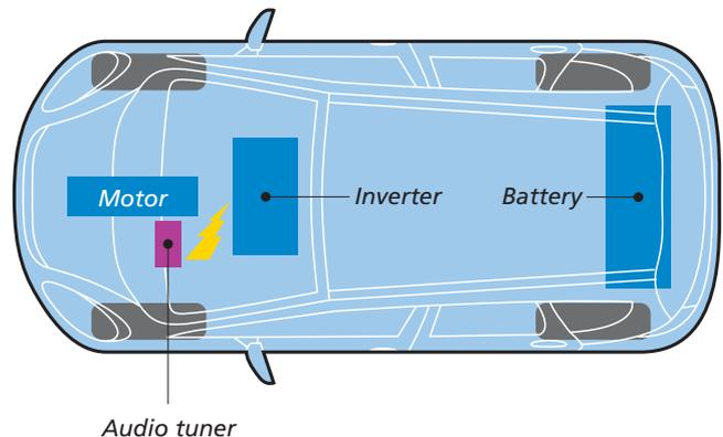
Example 3: Analysis of interference to broadcast radio caused by inverters of EV vehicles
