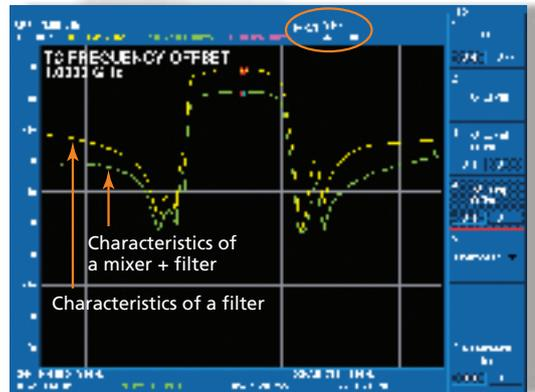
Measurement of mixer frequency conversion loss characteristics
