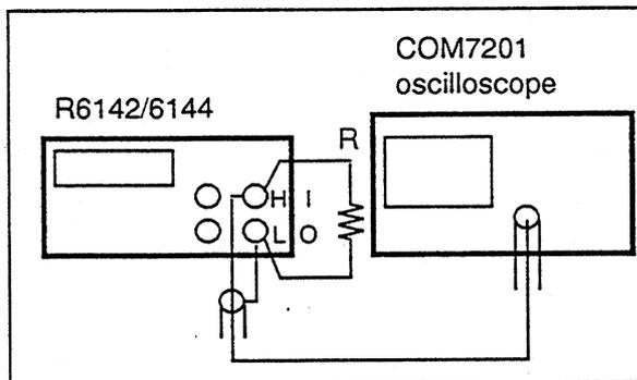
Figure 4-5 Cable Connection for High-frequency Noise Voltage Measurement
