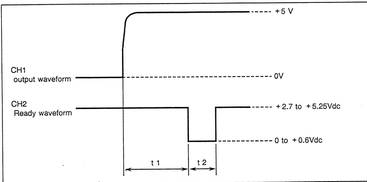
Figure 4-12 Waveform Timing
