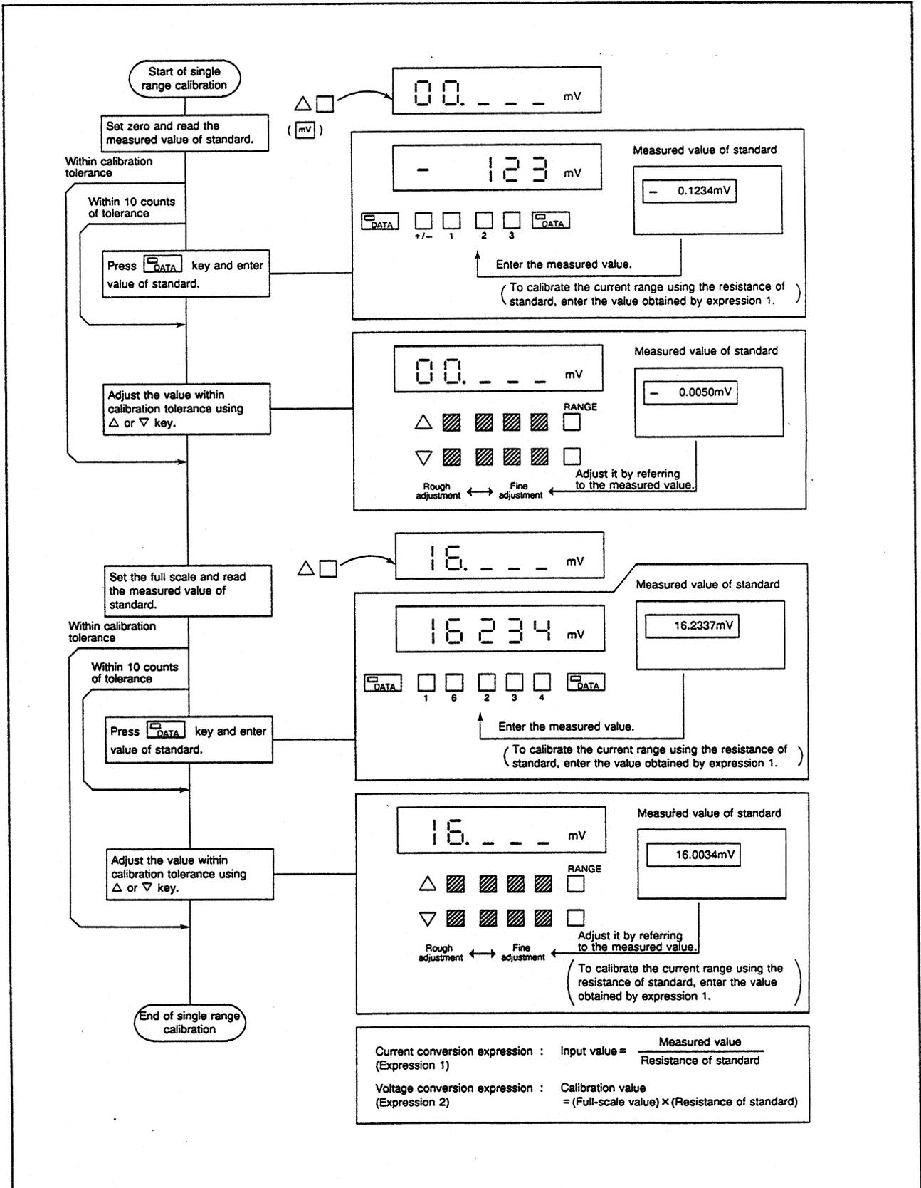
Figure 5-3 Calibration of A Single Range using R6144
