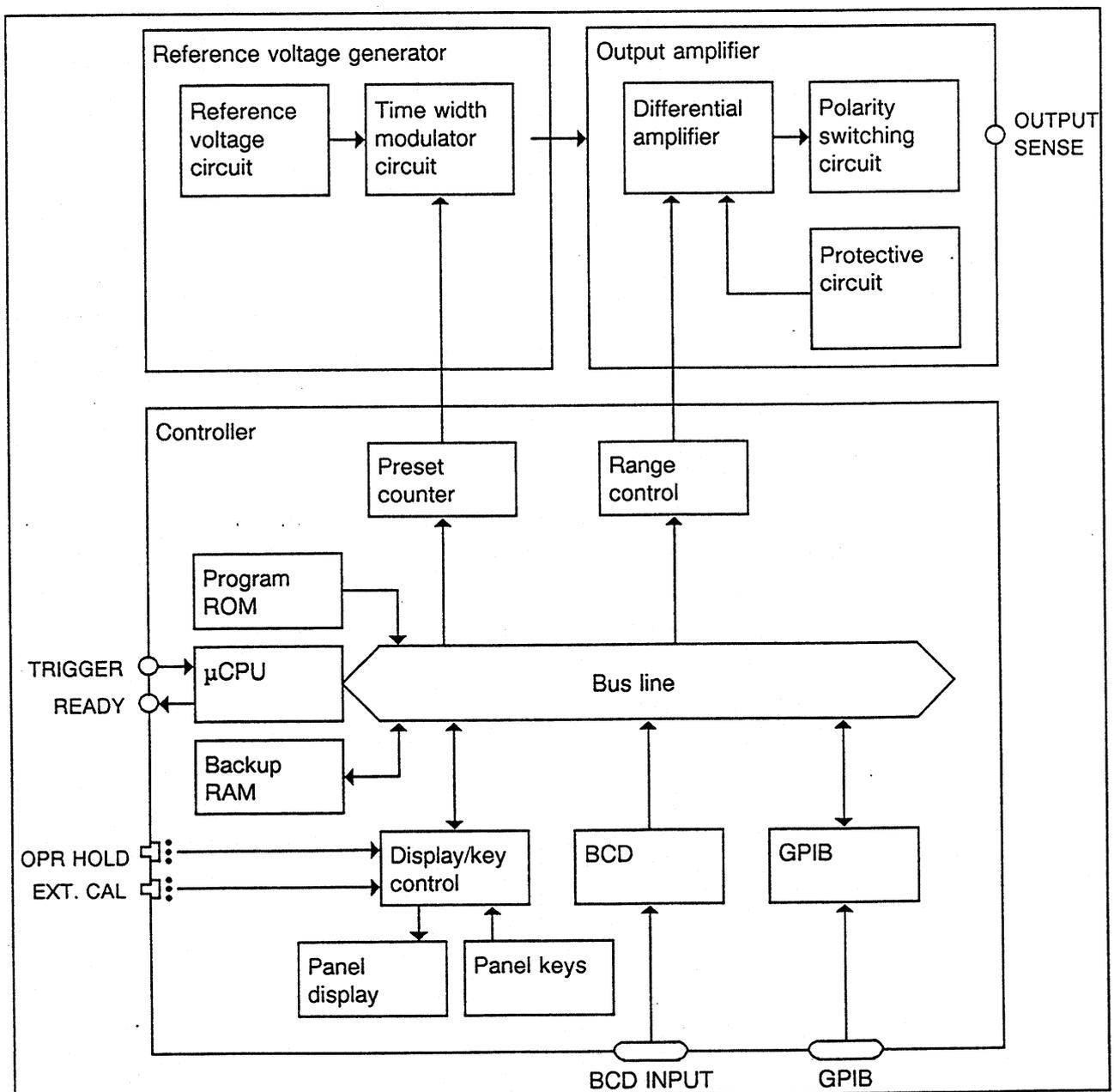
Figure 3-1 Block Diagram
