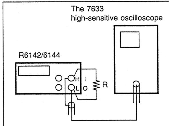
Figure 4-4 Cable Connection for Low-frequency Noise Current Measurement
