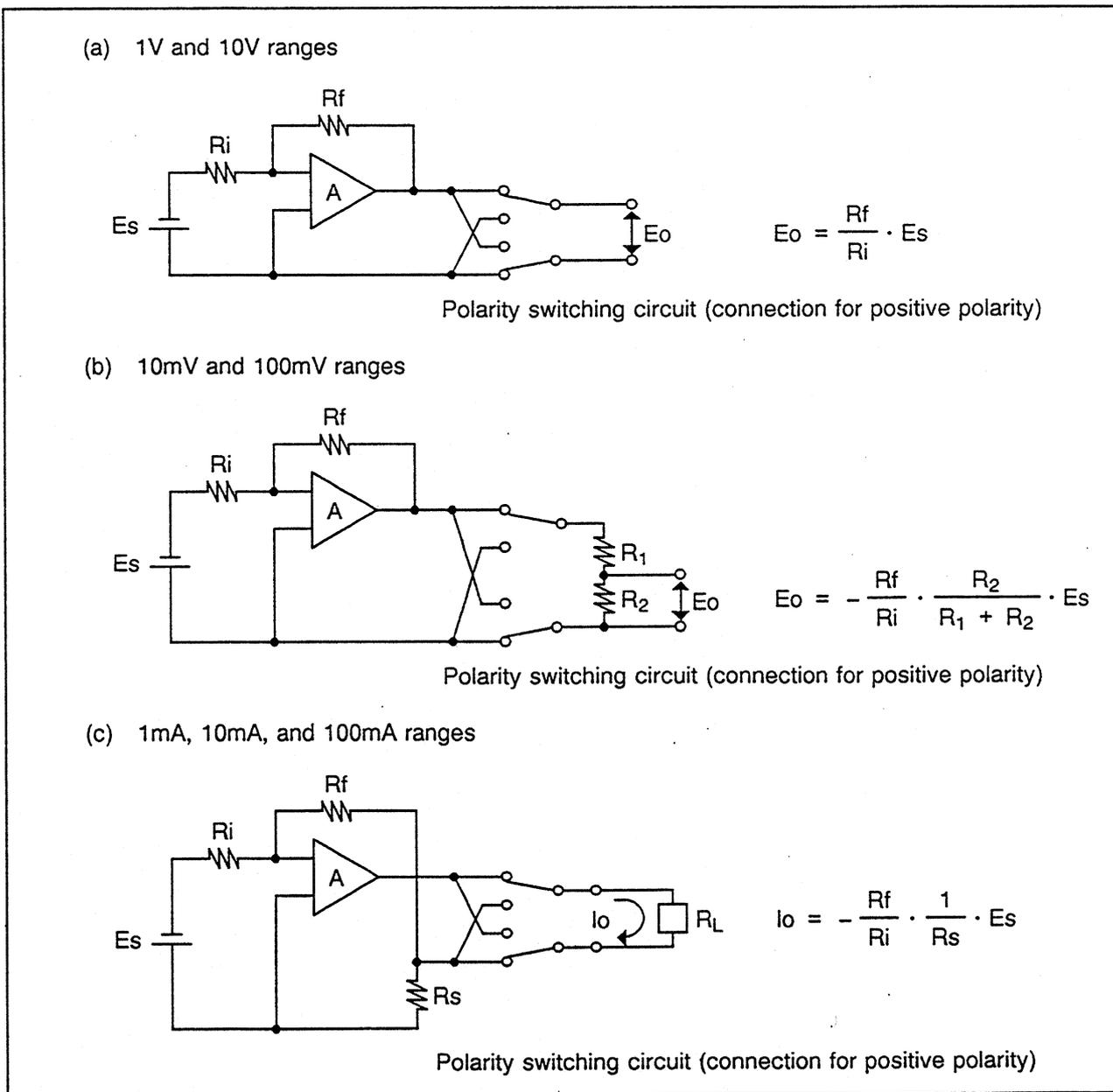
Figure 3-3 Principle of the Output Amplifier and Polarity Switching Circuit
