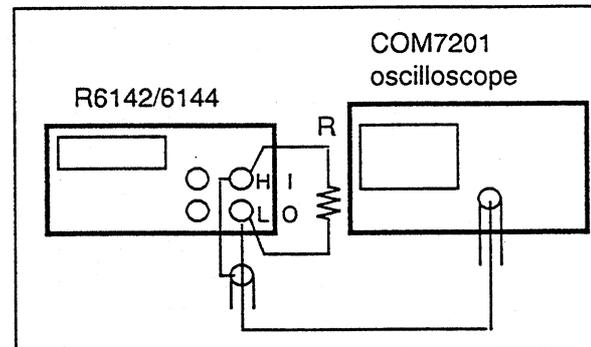
Figure 4-6 Cable Connection for High-frequency Noise Current Measurement
