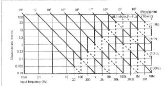
Maximum resolution: MSD 1 to 2: 9-digit display MSD 3 to 9: 8-digit display (resolution up to 0.1 mHz)
