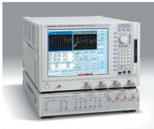
Combination with the R3968 multi-port test set
