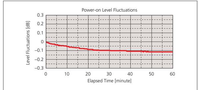
*Less fluctuation after power-on*
