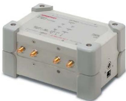
The high-impedance differential IQ signal converter circuit, which is independent from the R3671/3681 signal analyzer, can be placed close to the target device. The high-impedance signal line between a DUT and the measuring device can thus be shortened, and this reduces adverse effects on modulation precision by stray capacitance on the signal line and differences in line length.
