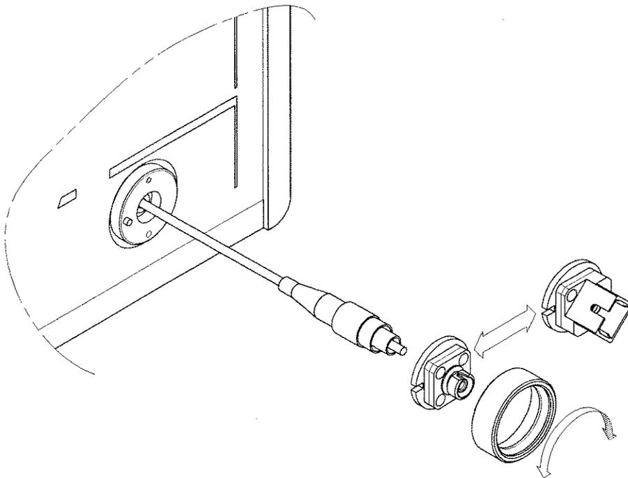
**Figure 1-4 Replacing/Cleaning Optical Connector-adapters for the Q8326**
