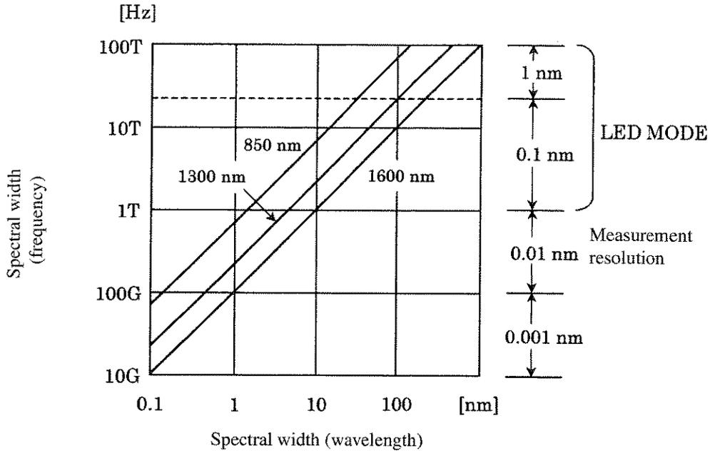
**Figure 2-4 Relationship between Spectral Width and Measurement Resolution**
