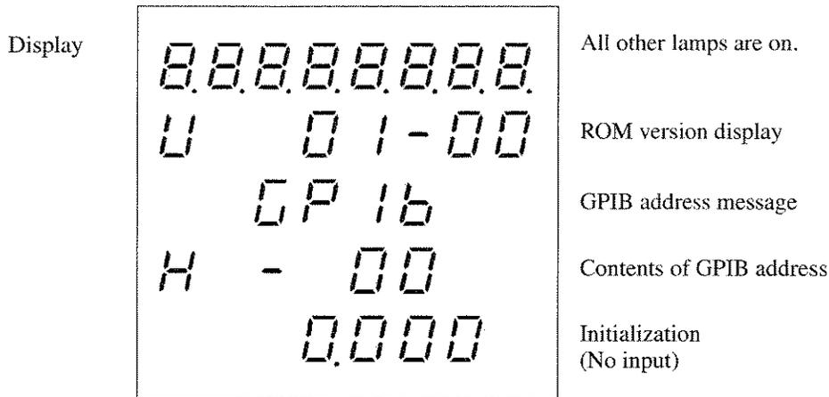
Figure 2-3 Panel Display after Master Reset
