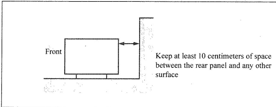
**Figure-2 Instrument Placement**
