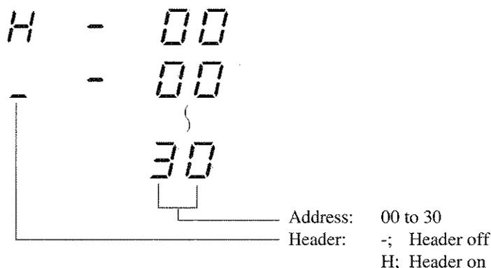
First, since the header is blinking, press the  $\leftarrow$  ( $\uparrow$ ) key to set the header on or off. After the header has been set, press the  $\rightarrow$  ( $\rightarrow$ ) key to set the address.
