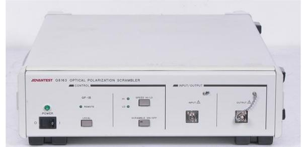
The Q8163 is an optical polarization scrambler which has a function to change the state of output light polarization with using a polarization element of optical fiber type. The state of output light polarization can be changed continuously by driving 3 polarization elements of optical fiber type. Therefore, all the states of polarized light (all the points on the Poincare sphere) can be output.
