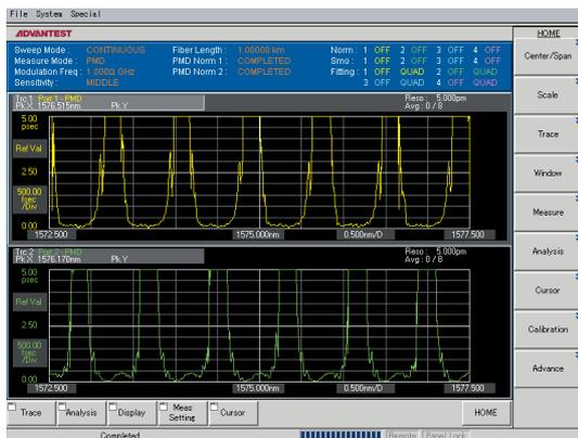
*PMD characteristics of interleavers (2-port measurement)*
