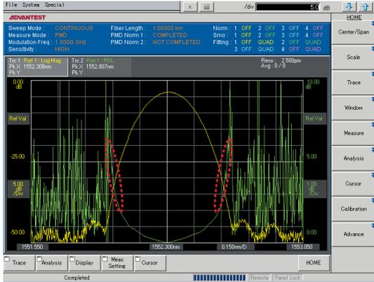
*IL/PDL characteristics of AWG*
