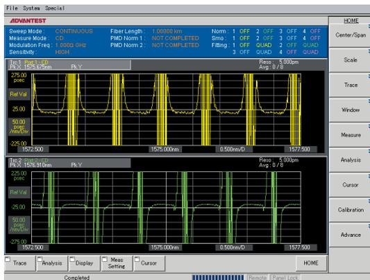
*CD characteristics of interleavers (2-port measurement)*
