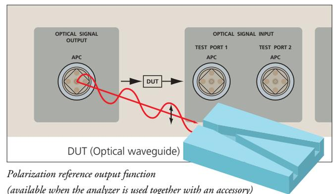
Polarization reference output function
