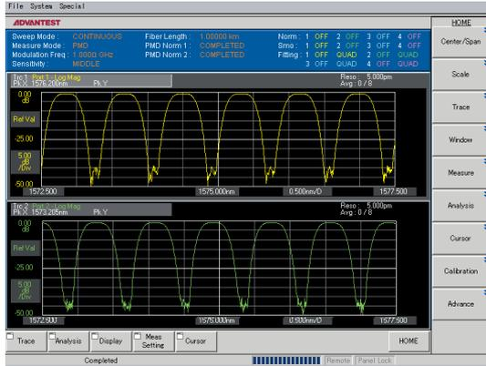
*IL characteristics of interleavers (2-port measurement)*
