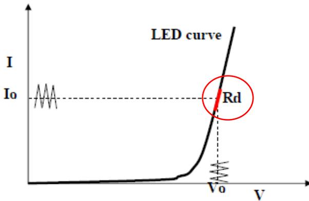
Figure 12 LED test by traditional electronic loads
