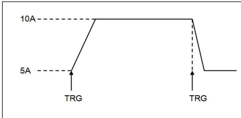
Figure 11 Dynamic test in toggle mode
