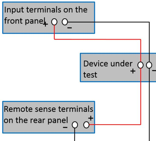
Figure 16 Remote sense connection
