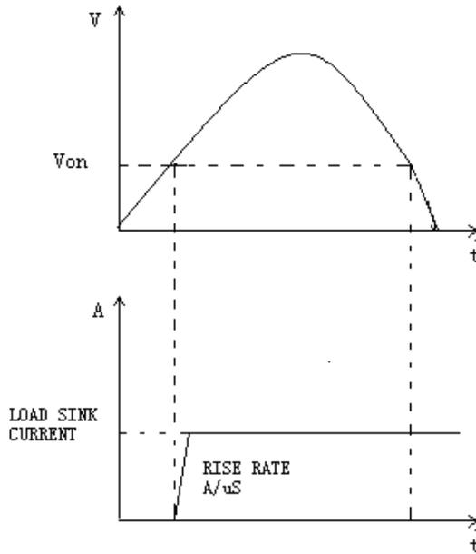
Figure 14 Load working range with Von latch enabled
