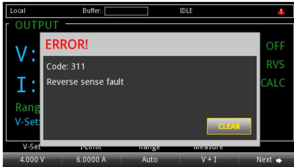
To clear the error, you need to clear the Questionable Instrument Summary Event Register bit and initiate the trigger model using the front panel or SCPI commands. For more information on registers, refer to [Questionable Instrument Summary Event Register](#) (on page D-16).
