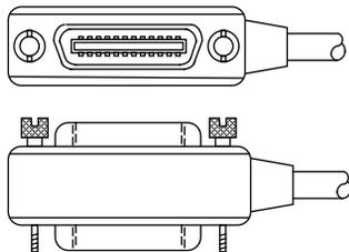
To allow many parallel connections to one instrument, stack the connector. Two screws are located on each connector to ensure that connections remain secure. Current standards call for metric threads, which are identified with dark-colored screws. Earlier versions had different screws, which were silver-colored. Do not use these types of connectors on the Model 2010 Multimeter, because it is designed for metric threads.
