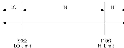
The CALC3:LIMit2 subsystem has all the same commands available as the CALC3:LIMit[1] subsystem. From the front panel, the same menu is used to control the beeping state and conditions (inside or outside) for both limits. Since there is only one beeper, there are two distinct tones used for the two limits, but limit set 1 will take precedence.
