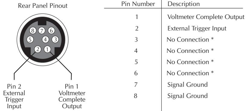
\* Either pin 3 or 5 may be configured as an output instead of pin 1. Either pin 4 or 6 may be configured as an input instead of pin 2. See the Model 2010 Service Manual for details.
