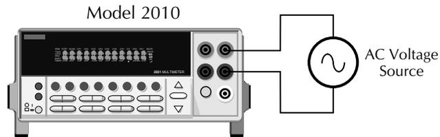
Input Impedance =  $1\text{M}\Omega$  in parallel with  $<100\text{pF}$
