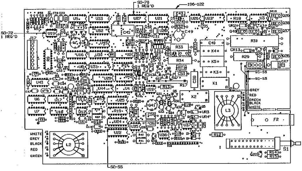
Figure 7-5. Analog Board, Component Location Drawing, Dwg. No. 196-120
