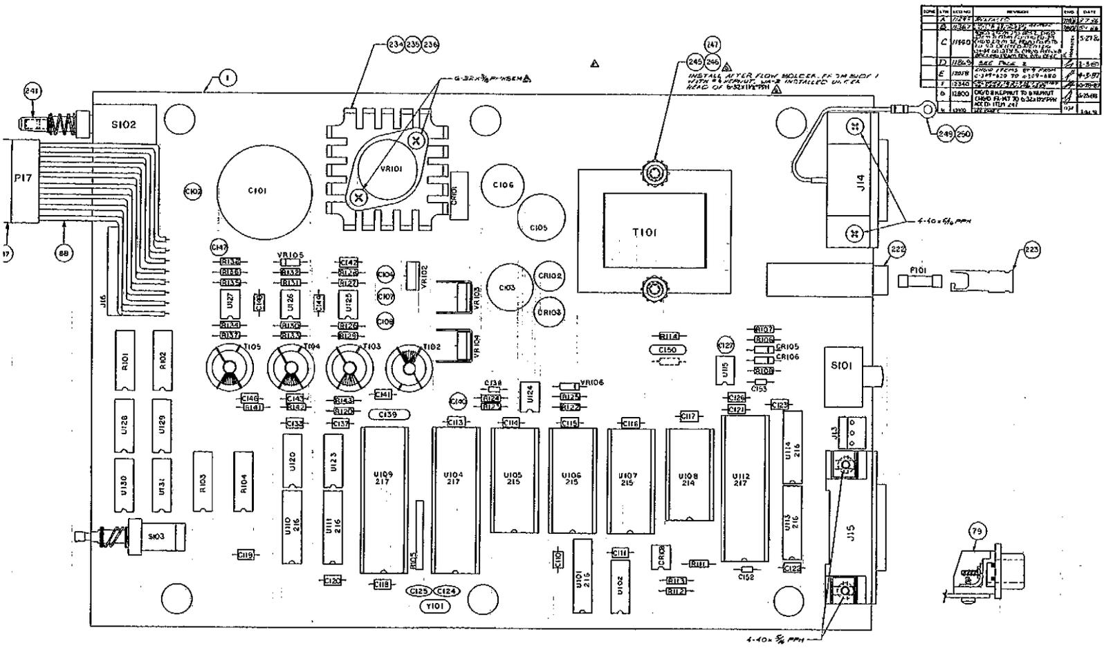
Figure 7-3. Digital Board, Component Location Drawing, Dwg. No. 196-100
