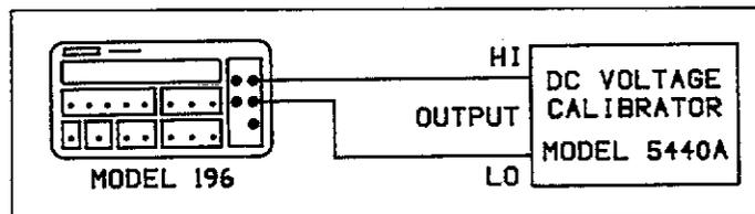
Figure 6-2. DC Volts Calibration Configuration (30V-300V Ranges)
