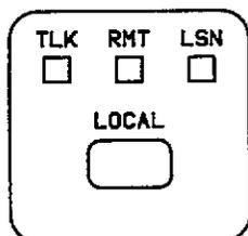
Since all front panel keys except LOCAL are locked out when the instrument is in remote, this key provides a convenient method of restoring front panel operation. Pressing LOCAL will also turn off the RMT indicator and return the display to the normal mode if user messages were previously displayed with the D command.
