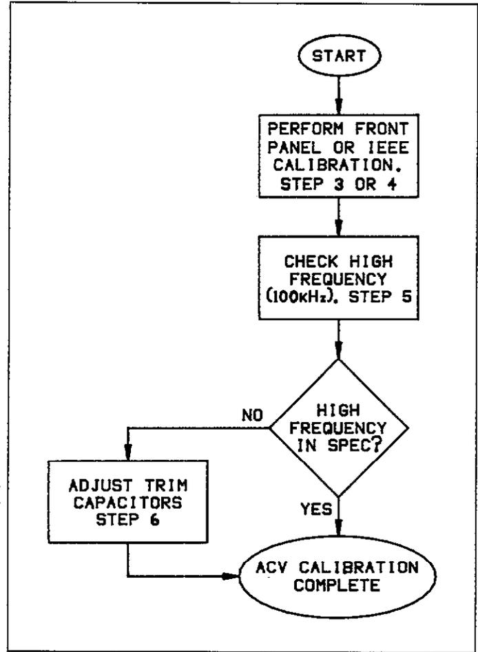
Figure 6-5. Flowchart of AC Volts Calibration Procedure
