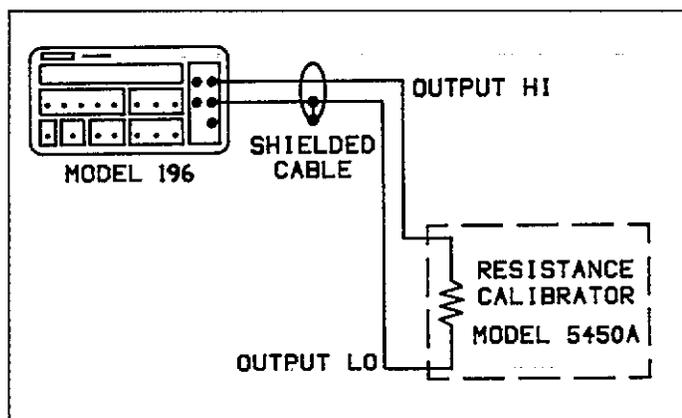
**Figure 6-4. Two-Wire Resistance Calibration Configuration (300kΩ-300MΩ Ranges)**
