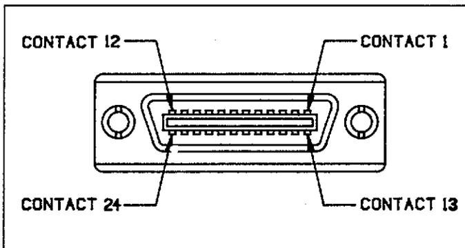
Figure 3-5. Contact Assignments
