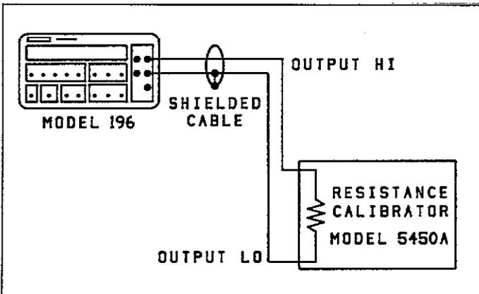
Figure 4-4. Connections for Ohms Verification (300kΩ–300MΩ Ranges)
