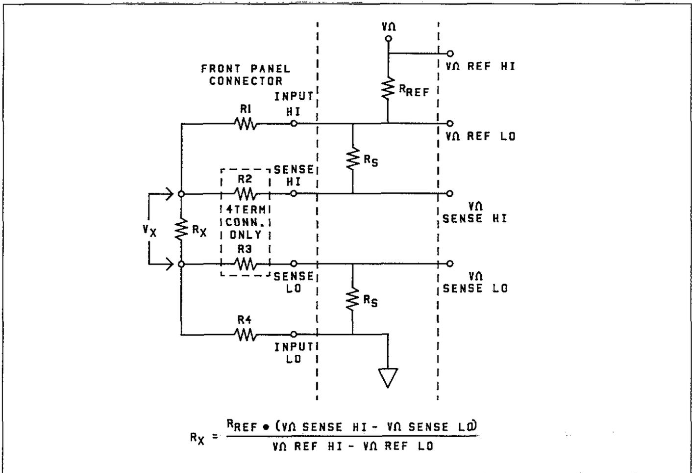
Figure 5-2. Input Configuration During 2 and 4-Terminal Resistance Measurement
