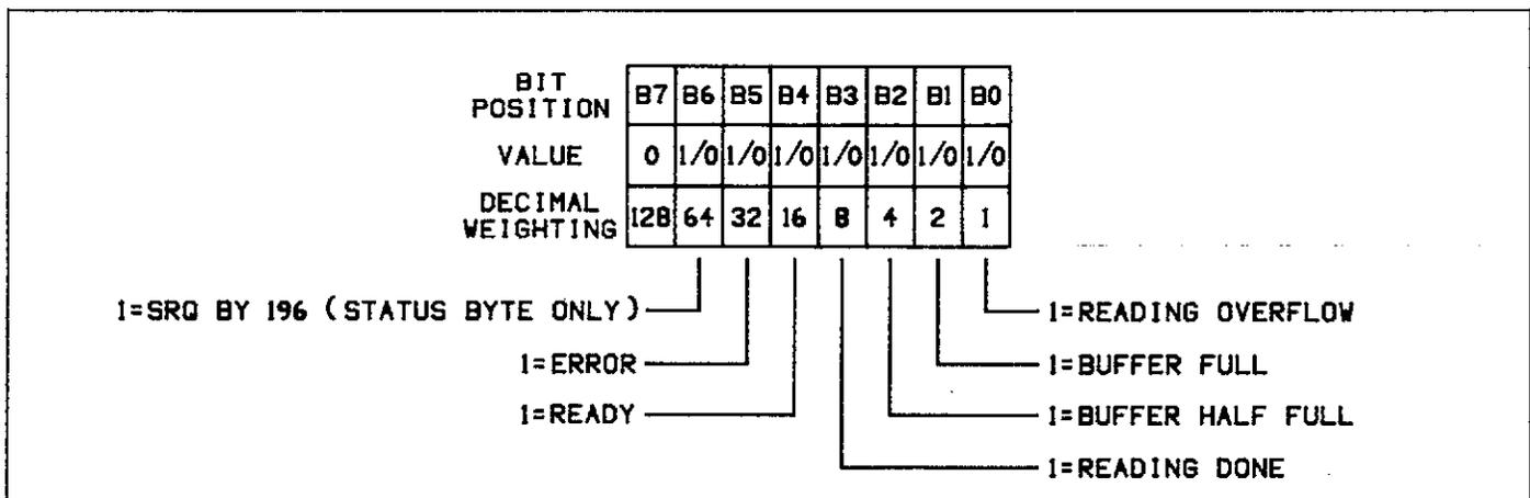
**Figure 3-7. SRQ Mask and Serial Poll Byte Format**
