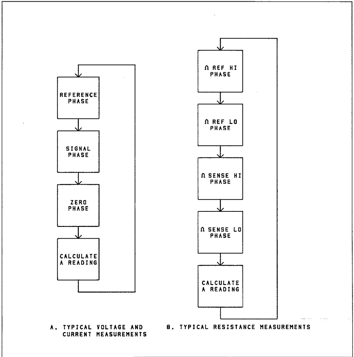
Figure 5-5. Multiplexer Phases
