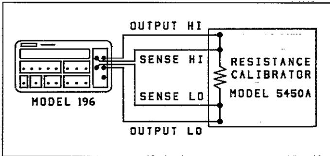
Figure 4-3. Connections for Ohms Verification (300Ω–30kΩ Range)
