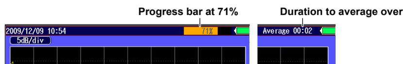
Measured data can automatically be saved when averaged measurements are completed. For the setup procedure, see section 3.5.
