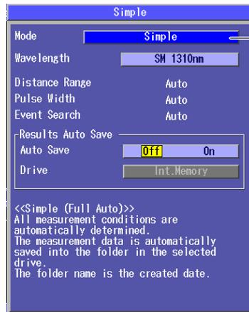
Set the measurement mode (Simple, Detail, Multi WL, PON). The Multi WL option is not available on the AQ1200B and AQ1200C.
