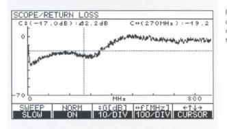
Frequency-dependent measurement of return loss using external SWR bridge
