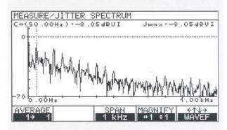
Output signals switched for jitter measurement to clock extractor method
