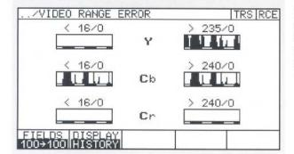
Measurement of standard-level infringements: display of too high levels (right) and too low levels (left)
