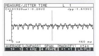
Jitter display in frequency spectrum, in example shown up to 1 kHz
