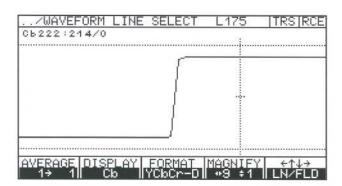
VCA combines the advantages of digital and analog measurements. Digital signal processing enables data storage and subsequent analysis of individual video lines. After switching on a digital filter with analog characteristic
