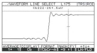
(right), the signal can be assessed and analyzed in detail. The example shows that too low signal rise time produces transients.
