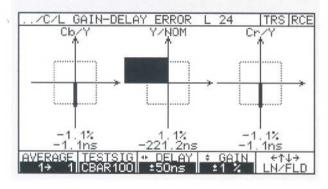
Level and delay measured with colour bar signal. Signal shown in example is three clocks too early (approx. 222 ns), luminance level is 1.1% above nominal value
