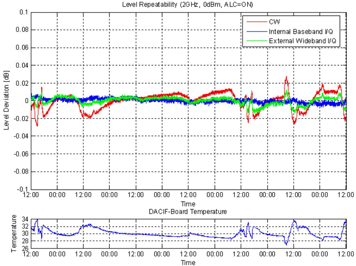
*Measured level repeatability over 6 days with random settings between measurements
