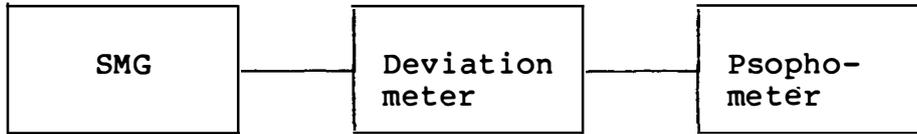
**Test:** Measure the residual FM with a CCITT weighting filter or unweighted (30 Hz to 20 kHz) and an RMS rectifier.
