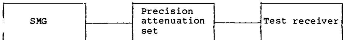
Ensure that the cable connections are RF tight.
