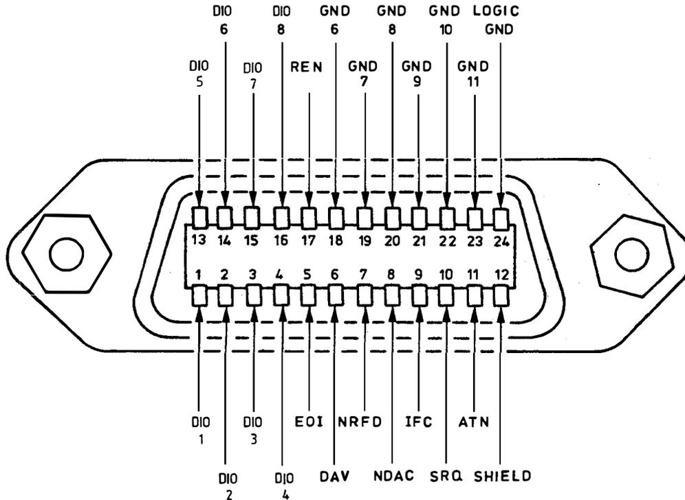
Fig. 2-13 Pin assignments
