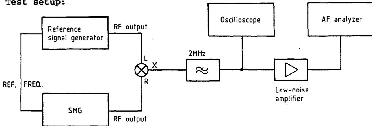
Synchronize the reference frequencies from the SMG and the reference signal generator.
