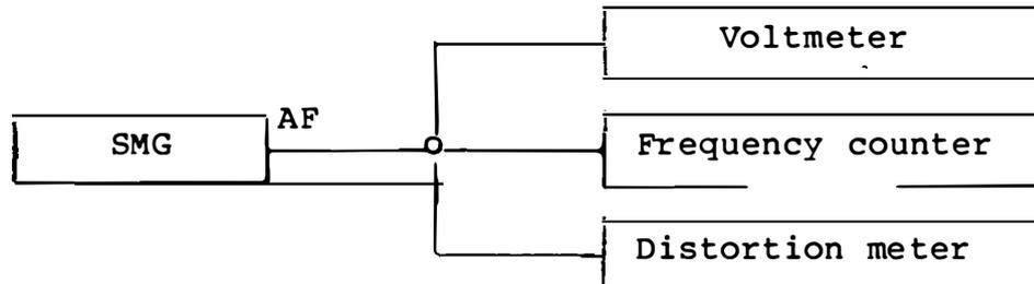
**Test:** Vary the frequency of the modulation generator from 40 Hz to 15 kHz (10 Hz to 100 kHz) and measure the level, frequency and distortion.
