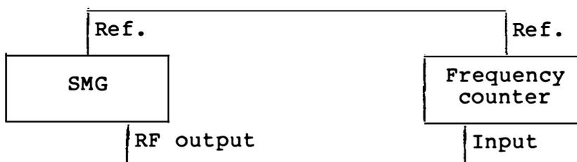
Synchronize reference frequency from SMG and from frequency counter.
