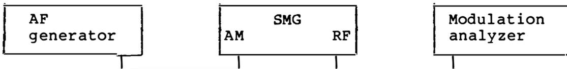
**Test:** Set a level of 1 V on the AF generator and vary the frequency from 10 Hz to 50 kHz.
