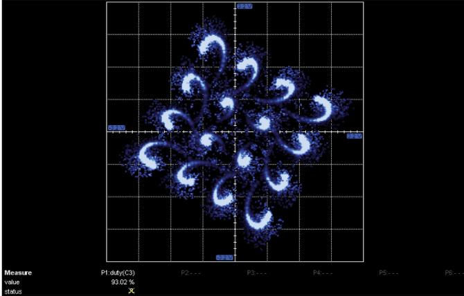
Fading spectrum with DVB 20 paths fading profile RL20ANxB.
