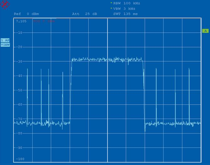
Useful signal with additive white Gaussian noise (AWGN).
