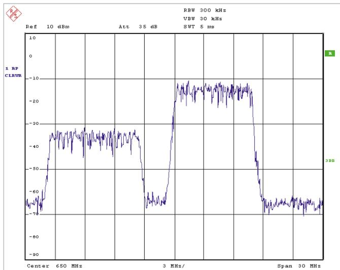
The R&S®SFU is the only broadcast signal generator that allows simulation of the digital dividend using only one instrument. The support of R&S®WinIQSIM2™ makes it possible to generate a large number of wireless communications standards with user-configurable waveforms, such as Long Term Evolution (LTE). The wireless communications standards can be added as interferers to the broadcast standards, which are available in realtime on the R&S®SFU, in order to simulate the desired scenarios.
