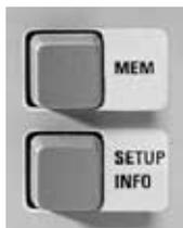
Information on the hardware and firmware configuration of the SFM is called up with the SETUP INFO key. Via this key, the parameters for the RS-232-C and IEC/IEEE-bus interfaces can be set, and the RF frequency resolution, level unit and type of 10 MHz synchronization can be selected.
