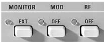
When fast tests are to be carried out, the IF modulation can directly be switched off and on with MOD OFF and the RF carrier with RF OFF without the associated submenu being opened.
