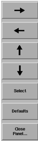
The **arrow** softkeys allow you to navigate from field to field in the dialog box. The highlighted parameter can be changed.
