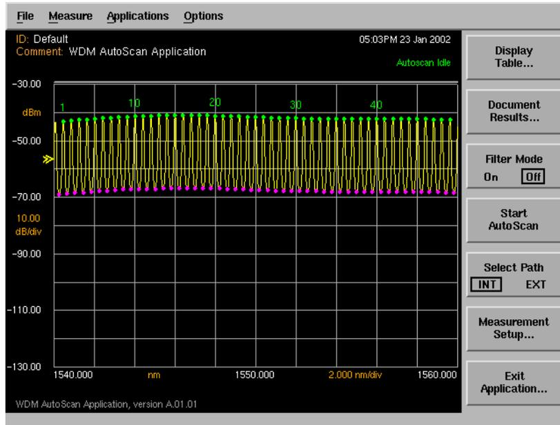
An automated channel scan is performed. The channel power, wavelength, optical signal-to-noise ratio, spectral gain tilt, and other statistics can be displayed either graphically or in a tabular format.
