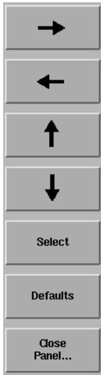
The **arrow** softkeys allow you to navigate from field to field in the panel. The highlighted parameter can be changed.
