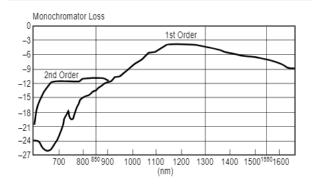
\*Second order is selected when the stop wavelength is at or below 900 nm and resolution is <10 nm.
