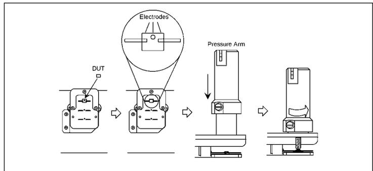
1. Align the DUT with the device guide and place it on the contact board.
