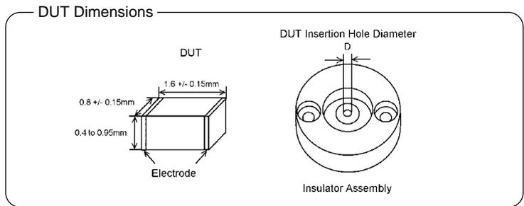
The 16196A is furnished with three different insulator assemblies, since any gaps between the DUT and the cylindrical insulator will result in improper positioning and subsequent measurement errors. Select an insulator assembly that reduces the gap the most. See the table below for dimensions of the insulator assemblies.
