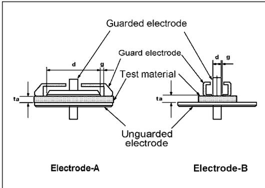
Electrodes for contacting electrode method
