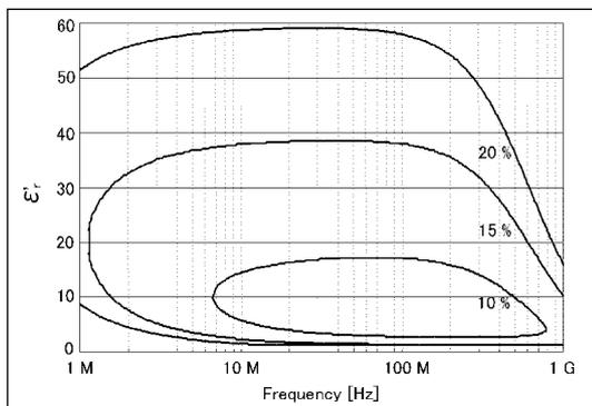
Typical Permittivity ( $\epsilon_r$ ) Measurement Accuracy (@ thickness = 1 mm)
