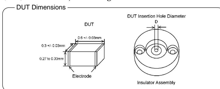
The 16196C is furnished with one insulator assembly. See the table below for the dimensions of the insulator assembly.
