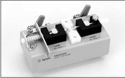
**Terminal Connector:** 4-Terminal Pair, BNC
