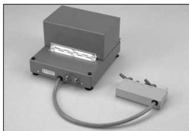
High Voltage BNC(f) connector for external bias input
