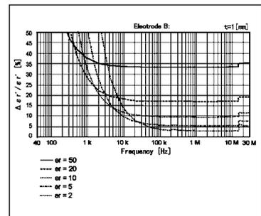
Typical Loss Tangent ( $\tan \delta$ ) Measurement Accuracy:
