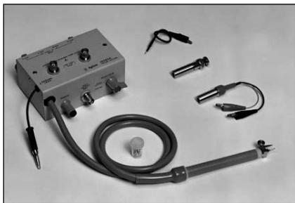
**Terminal Connector:** 4-Terminal Pair, BNC
