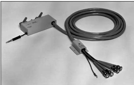
**Terminal Connector:** 4-Terminal Pair, BNC
