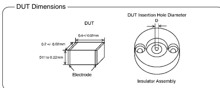
The 16196D is furnished with two different insulator assemblies, since any gaps between the DUT and the cylindrical insulator will result in improper positioning and subsequent measurement errors. Select an insulator assembly that reduces the gap the most. See the table below for dimensions of the insulator assemblies.
