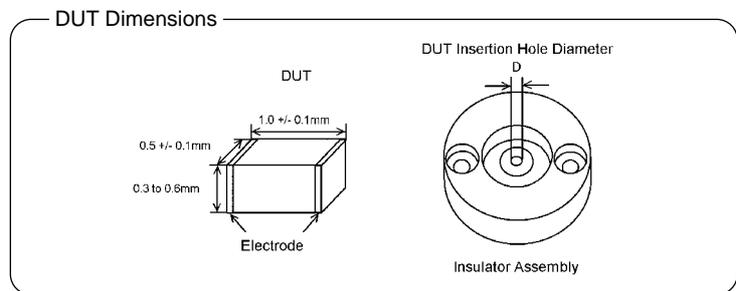
The 16196B is furnished with three different insulator assemblies, since any gaps between the DUT and the cylindrical insulator will result in improper positioning and subsequent measurement errors. Select an insulator assembly that reduces the gap the most. See the table below for dimensions of the insulator assemblies.
