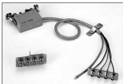
**Terminal Connector:** 4-Terminal Pair, BNC
