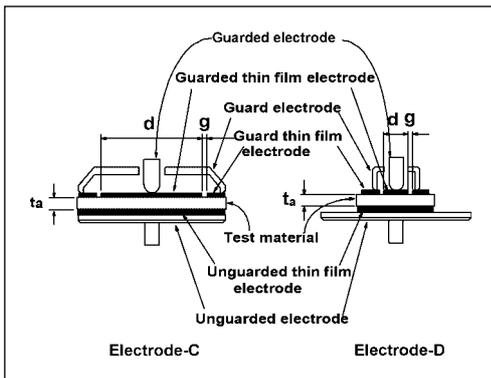
Electrodes for contacting electrode method
