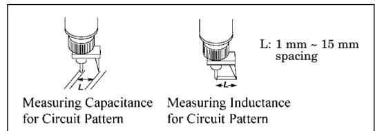
**Description:** 16094A is used along with the 7 mm cable (P/N 8120-4779). Together they provide the capability to perform in-circuit measurements (printed circuit patterns, the input/output impedance of circuits, etc.).
