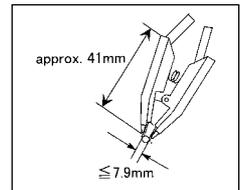
**Description:** The 16005C/D is useful when measuring test devices that have thin leads. It incorporates the Four-Terminal (Kelvin) connection method for accurate low resistance measurements. The jaws of the 16005C/D are a set of electrically independent contacts. The current terminal feeds the test current to the DUT while the voltage terminal detects the voltage across the DUT. Furthermore, the contact design assures accurate measurement down to the lowest resistance range.
