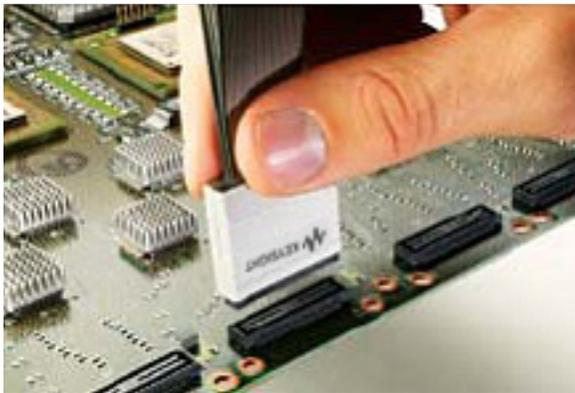
E5385A 34-channel Samtec connector probe
