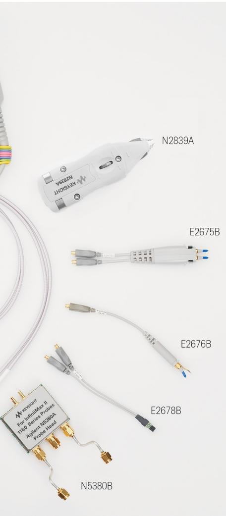
N2839A 12-GHz browser provides the measurement fidelity of a solder-in head to hand-held browsing with extremely low loading. The spring-loaded pogo tips ensure a secure connection and the tips can be adjusted from 0 to 3 mm apart. The tips can be easily replaced if accidental damage occurs.
