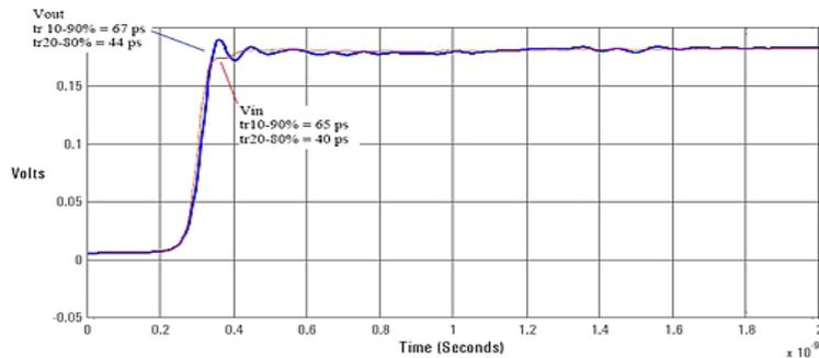
Graph of Vin and Vout of 1169B and N5381B solder-in head with a 25  $\Omega$  58 psec step generator
