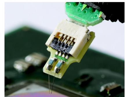
N2887A InfiniiMax Soft touch Pro Probe Adapter adapts from the Keysight Pro Series (36 ch) Soft touch connectorless logic analyzer foot print to the Keysight InfiniiMax I and II Series probe amplifier input connectors.
