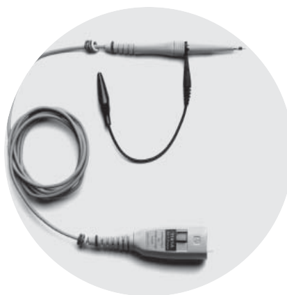
Figure 2.2. Agilent 116XA general purpose passive probe.
