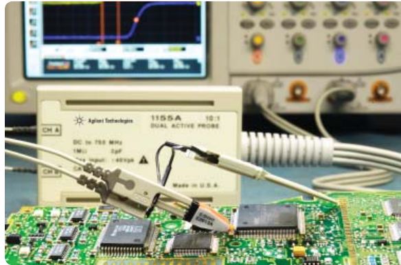
Figure 3.6. Agilent Wedge Probe Adapter for reliable, hands-free probing of 0.5 mm ICs.
