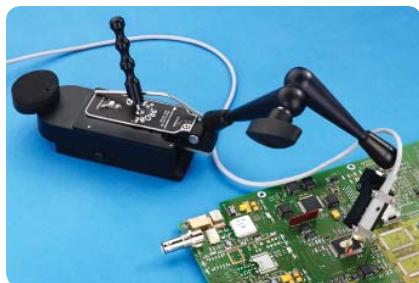
Figure 9.4. A fully articulated arm allows positioning in a variety of applications.
