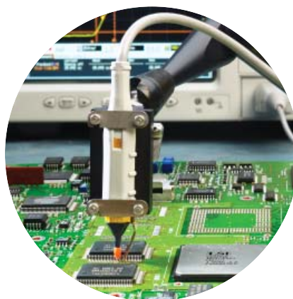
Figure 3.2. Agilent 1156A/57A/58A active probes for signals up to 4 GHz.
