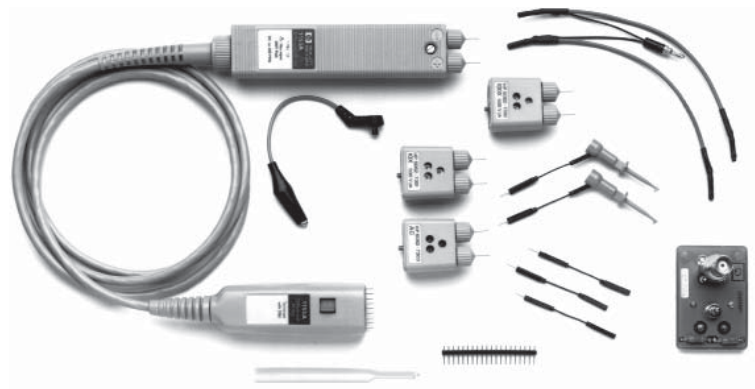
Figure 4.3. Agilent 1153A 1:1 FET differential probe with 200 MHz bandwidth.
